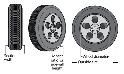
Figure 2—Measurements supplied for tire size information
