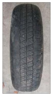
**Figure 13—**Underinflated tire The inside and outside edges are worn down; the middle is not. This is a telltale sign of underinflation.
