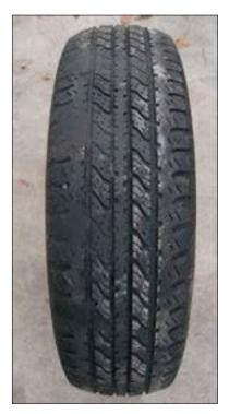
**Figure 12—**Cupping Cupping happens when worn or damaged suspension components cause the tire to bounce as it travels. Bad shock absorbers are the usual cause.
