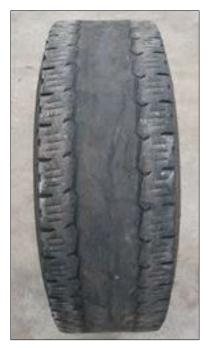
**Figure 10—**Centre wear The tire in Figure 8 was overinflated, causing the centre ring only to contact the road.
