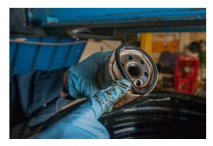
Figure 5—Make sure the old oil filter seal is removed with the filter.
