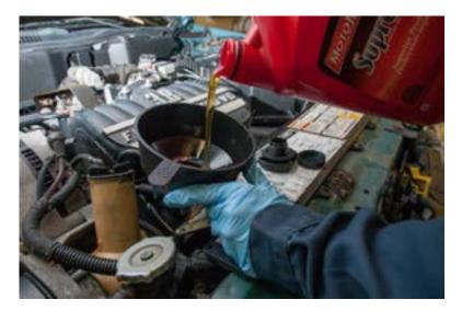
Figure 8—Fill engine oil
