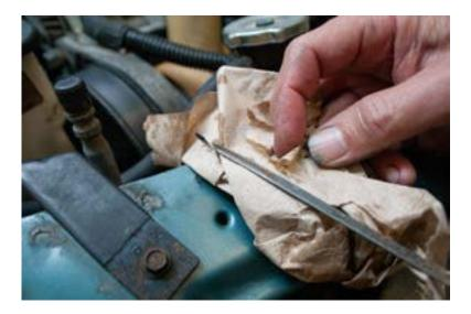
Figure 10—Check oil level using the oil dipstick
