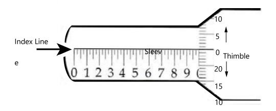
The **sleeve** does not move. It looks like a ruler with 10 numbers. The space between each number is divided into quarters. As the **thimble** rotates around this sleeve it covers up or reveals the numbers marked on the sleeve.
