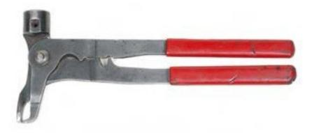
Figure 1—Wheel balance weight pliers
