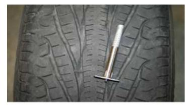
Figure 3—Directional tire with wear bar indicated; depth gauge indicates 5 mm depth reading.
