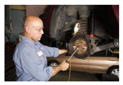
Figure 1—Wearing eye protection for a brake job
