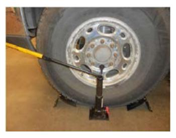
Figure 5—Using a pipe for additional leverage and the car jack as a fulcrum under the lug nut wrench
