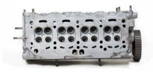
**Figure 10**—Bottom view of cylinder head showing where the valves sit **Note:** This has four valves per cylinder (two intake and two exhaust).
