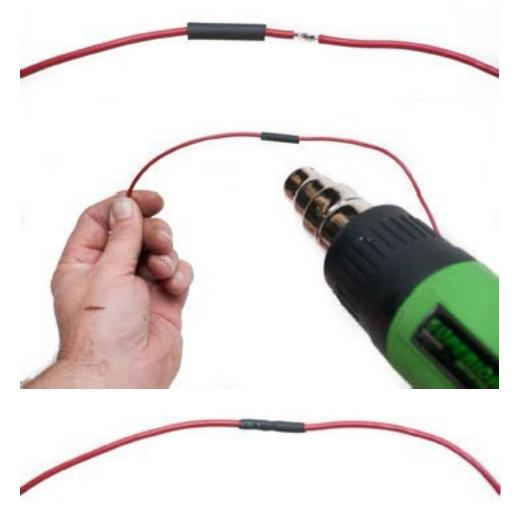
Figure 7—Applying heat shrink to a soldered joint
