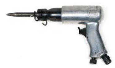
Figure 8—Air chisel
