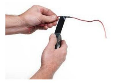
Figure 6—Finish by ending on the wire insulation on the other side.
