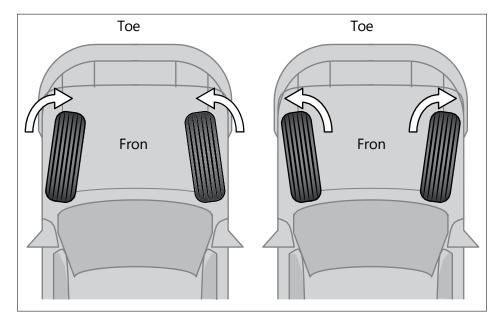
Figure 18—Toe in and toe out
