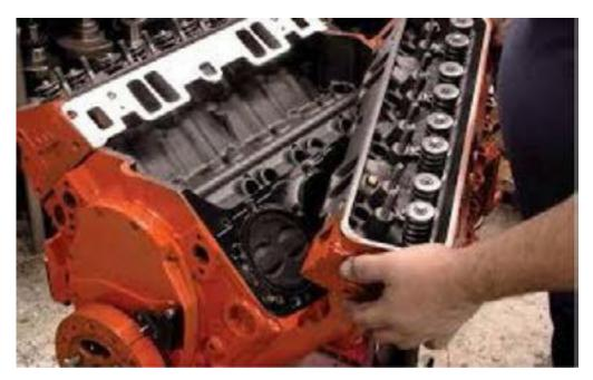
Figure 11—Cylinder head being attached to engine block
