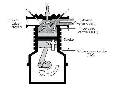
Figure 22—Exhaust stroke
