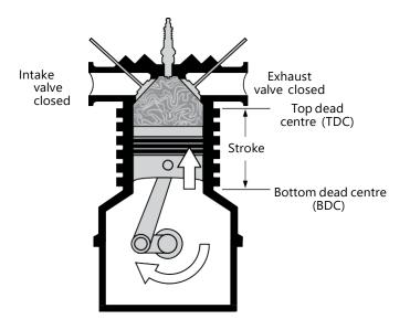
Figure 20—Compression stroke
