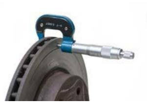
Figure 3—Measuring a brake rotor
