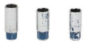
Figure 2—Spark plug socket
