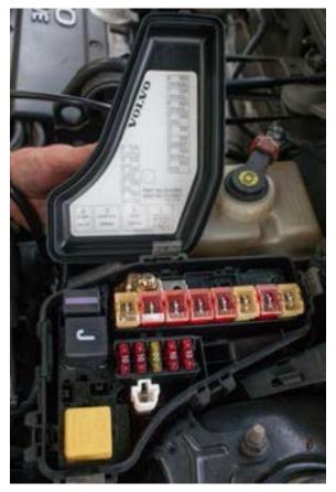
Figure 6—Typical fuel pump relay location
