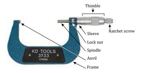
Figure 1—Micrometer parts
