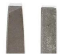
Figure 16—Files with tapered and blunt end
