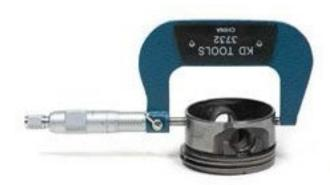
Figure 2—Measuring a piston
