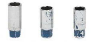
Figure 40—Spark plug socket wrench
