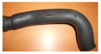
Figure 9—Clean and dry the hose about 2" on either side of the burst section
