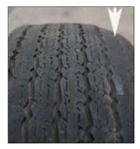
**Figure 15—**Camber wear With camber wear, the tire wears on one side only. This is usually a sign of the camber being out of adjustment.
