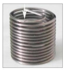
**Figure 6—**Inverted HeliCoil insert Note the notch at the tang's base, designed so the tang will break off more easily upon impact when struck with the tang breakoff tool
