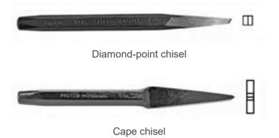
Figure 23—Types of chisels
