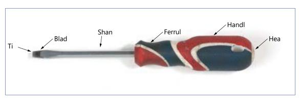
Figure 7—Parts of a screwdriver
