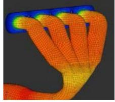
Figure 9—Thermal analysis of exhaust system and manifold. Hot exhaust can seriously burn you.
