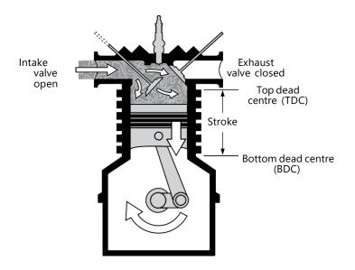
Figure 19—Intake stroke
