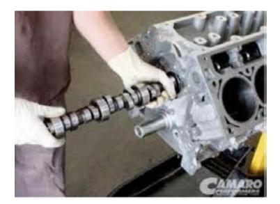
Figure 16—In-the-block camshaft
