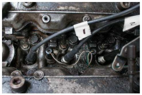
Figure 5—Spark plug wires attached to engine
