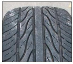
Figure 4—Siped directional tire
