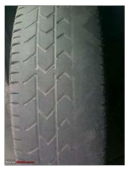
Figure 19—Tire wear from toe-in or toe-out
