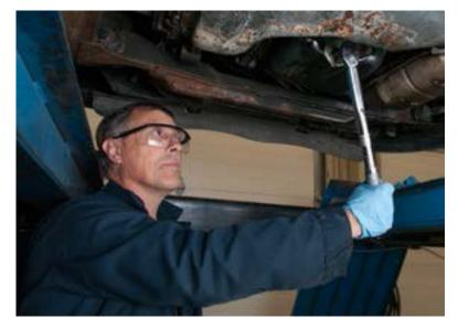
Figure 3—Use a torque wrench to tighten the oil drain plug.
