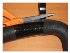
Figure 11—Cutting the electrical tape
