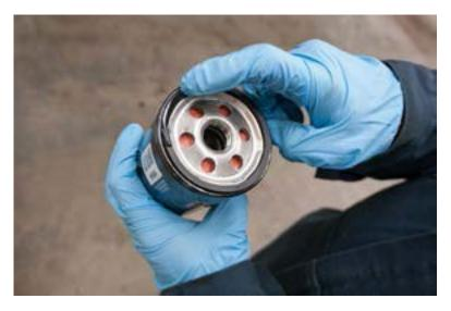
Figure 6—Lubricate the new oil filter seal
