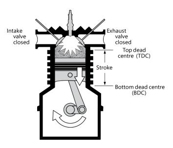
Figure 21—Power stroke
