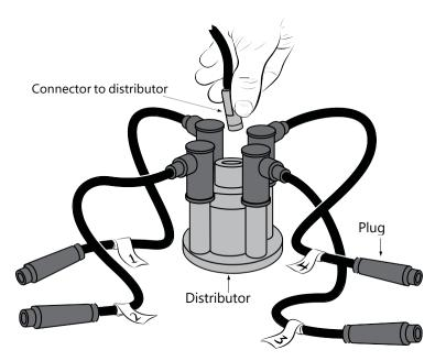
**Figure 7—**Label the spark plug wires so they do not get mixed up. Then remove the centre wire and ground this high-tension lead.
