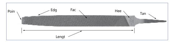
Figure 15—Parts of a file
