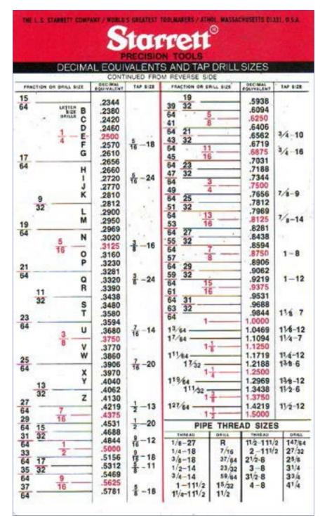
Figure 8—Example of drill bit size chart for imperial taps
