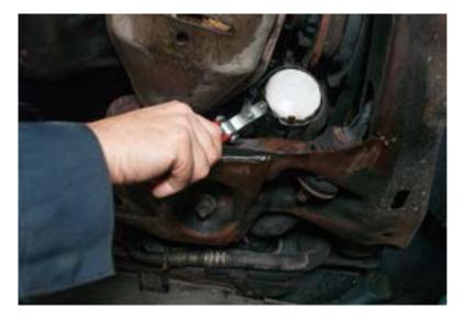
Figure 4—Remove oil filter
