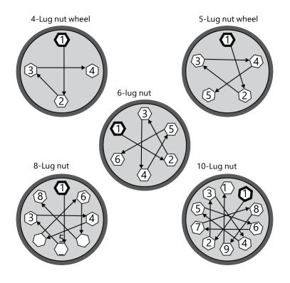
Figure 8—Wheel nut lug torque sequence
