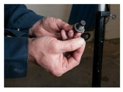
Figure 2—Drain plug seal
