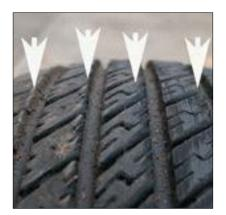
**Figure 14—**Feathering Feathering happens when a vehicle has a Toe In or Toe Out alignment issue. Note the slanted wear and high points on the edge of each row of tread
