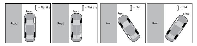
Figure 1—Positioning a vehicle with a flat tire to block any traffic from hitting the person changing the tire while changing it
