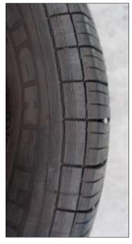
**Figure 11—**Cracking and bulging Cracking and bulging usually comes from hitting a pothole, curb or from an older tire.
