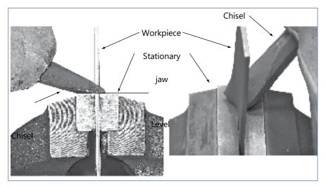
Figure 24—Correct use of chisel
