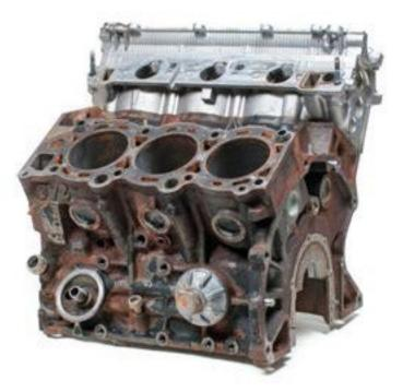
Figure 1—Cylinder block with head attached
