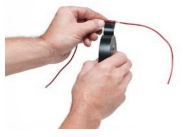
Figure 5—Wrap the solder joint by looping the tape securely.
