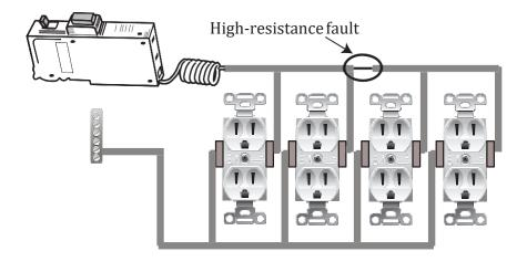
**Figure 6**—Circuit with high-resistance fault. In this example there is a high-resistance fault between the 2<sup>nd</sup> and 3<sup>rd</sup> receptacle. The voltage drop increased from the 2<sup>nd</sup> to the 3<sup>rd</sup>. The high resistance was identified as a poor connection between the two devices.
