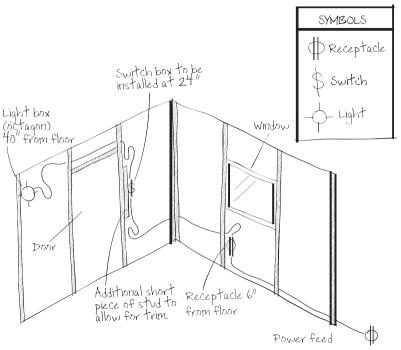
Figure 6—Sketch of wired wall section
