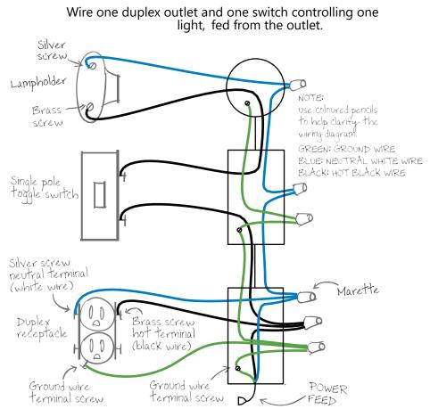
Figure 7—Wiring diagram of circuit
