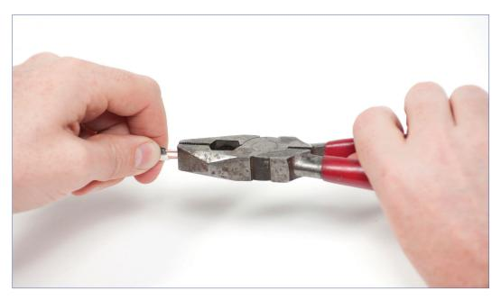
Figure 2—Twist the two wires together
