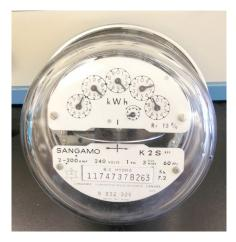
Figure 2—Kilowatt-hour meter
