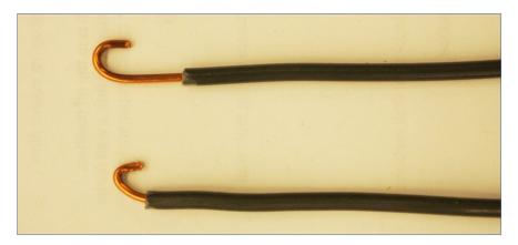
Figure 21—Bad hooks (too little insulation stripped and too much stripped)
