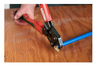
Figure 14—Using the crimping tool
