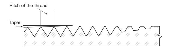
Figure 10—Close-up of tapered pipe threads
