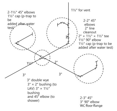
Figure 24-Rough in isometric
