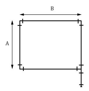
Figure 9—Copper loop. Adapter is soldered on for pressure test.
