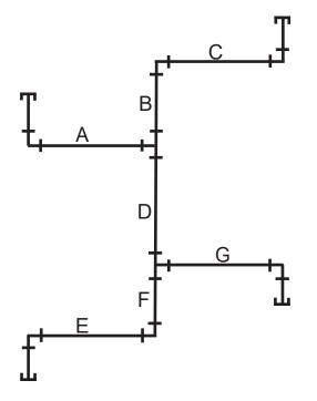
Figure 12—Piping system for threading project
