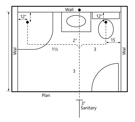
Figure 23—ABS rough-in (key)
