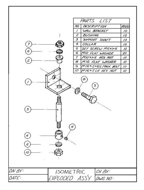
Figure 16—Assembly drawings are typically drawn in isometric form, as they can convey how parts are to be connected.
