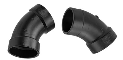
**Figure 3**—ABS 45°. The hub by hub 45 shown on the left connects two pieces of piping. The hub by spigot 45 shown on the right fits directly into another fitting (typically a wye).
