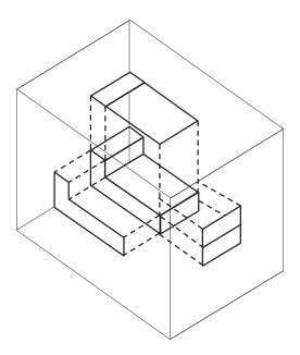
Figure 4—Each side of the glass box shows only one plane of the object, and all lines are straight and parallel.
