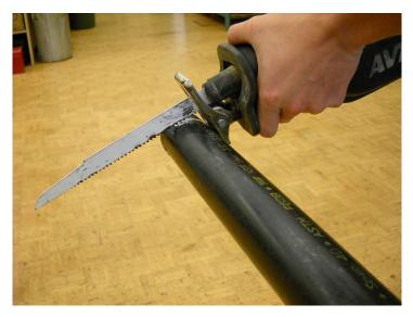
Figure 18—Reciprocating saws cut ABS pipe very quickly.
