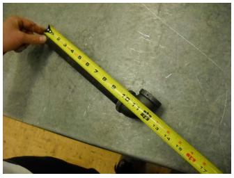
Figure 6—Correctly taking an end-to-centre measurement.
