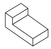
Figure 15—Isometrics show a three-dimensional object from three perspectives in a single drawing.
