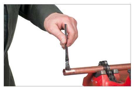
Figure 6—Flux will allow the solder to freely flow around the pipe.
