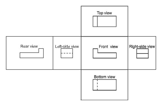
Figure 6—Drawing with the glass box flattened out
