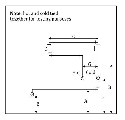
Figure 19—Crimping rough-in: front view
