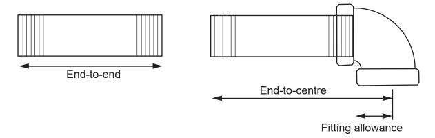
Figure 4-End-to-end, end-to-centre, and fitting allowance
