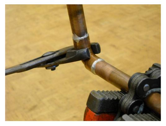
Figure 8—Copper fittings should be grasped at the corner so they don't bind on the pipe.
