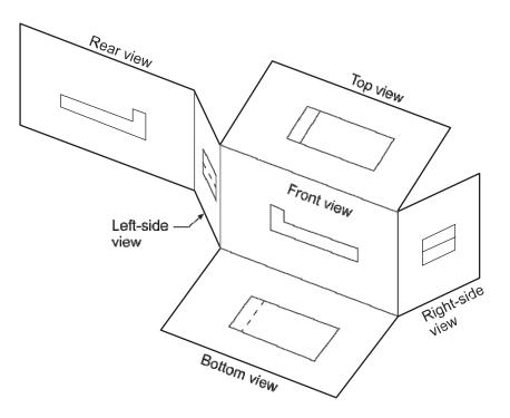
Figure 5—Views in an orthographic drawing
