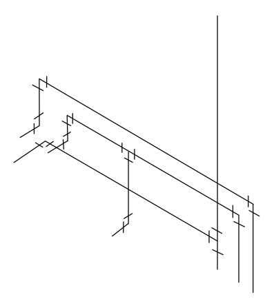
Figure 25—Isometric drawing of drainage and water lines
