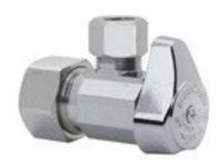
**Figure 6**—A compression-style CR 19 will fit over copper pipe. The chrome nut is then tightened to compress a brass ring, providing a watertight seal.
